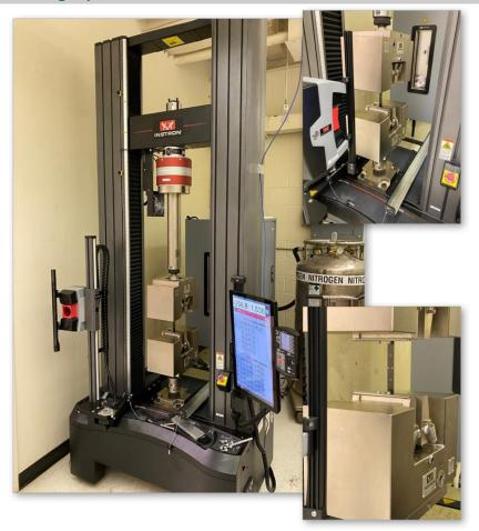
DatapointLabs announces expanded capability for the testing of structured composites, with the installation of a new 250 KN Instron UTM with environmental chamber and full video/DIC capability. The new NADCAP-compliant machine can perform tests over a -60C to 200C temperature range. It is capable of testing high strength materials, such as unidirectional (UD) and woven carbon fiber (CFRP) composites.
