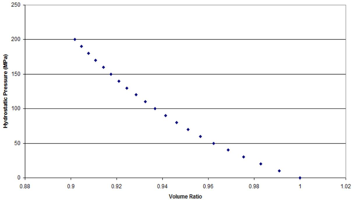
Figure 3 Stress v. Volume Ratio curve for the rubber
