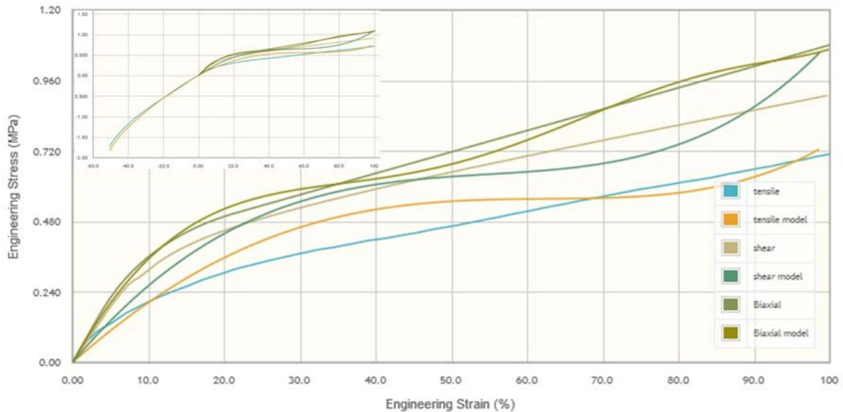
Figure 5 Mooney-Rivlin 9 Parameter model plot of both data and model (ANSYS fit)
