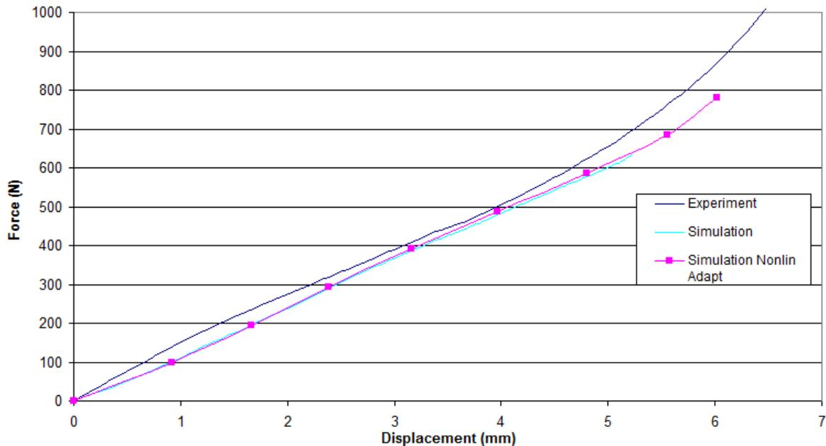
Figure 13 Comparing experiment force v. displacement to basic and adaptive mesh simulation
