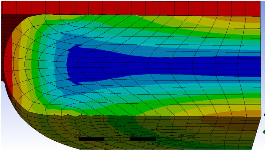
Figure 11 True-scale showing overlap in the button to upper platen and the distortion on button
