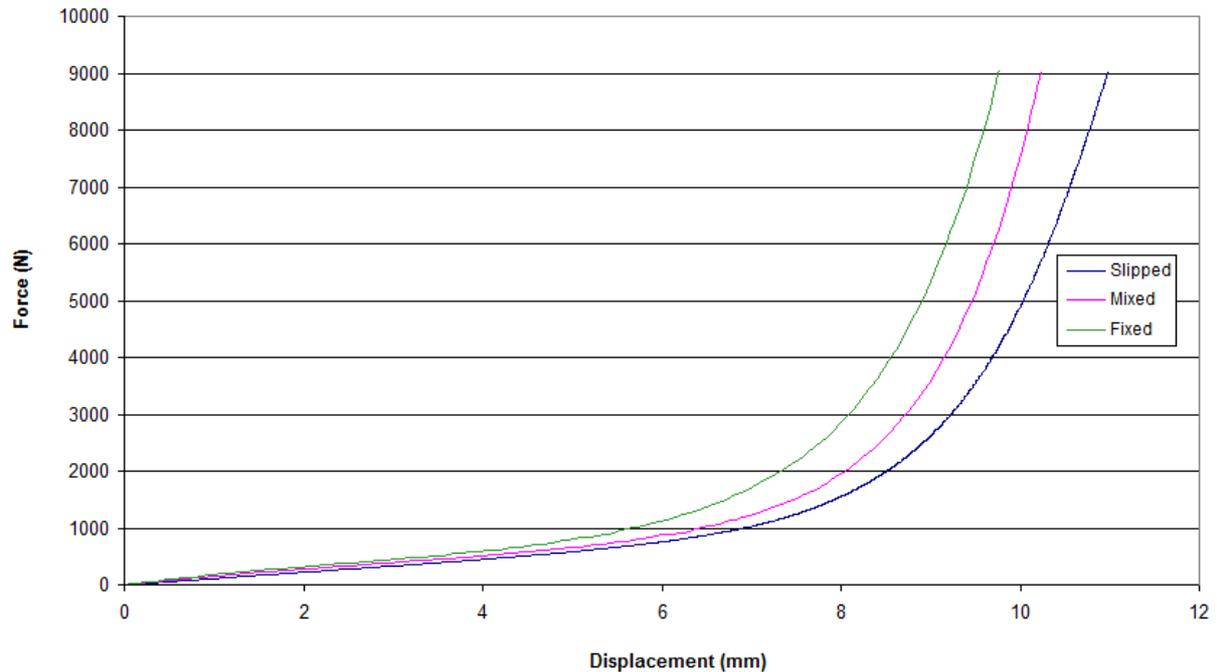
Figure 7 Force v. displacement curves for the compression tests with fixed, mixed, and slip boundary conditions
