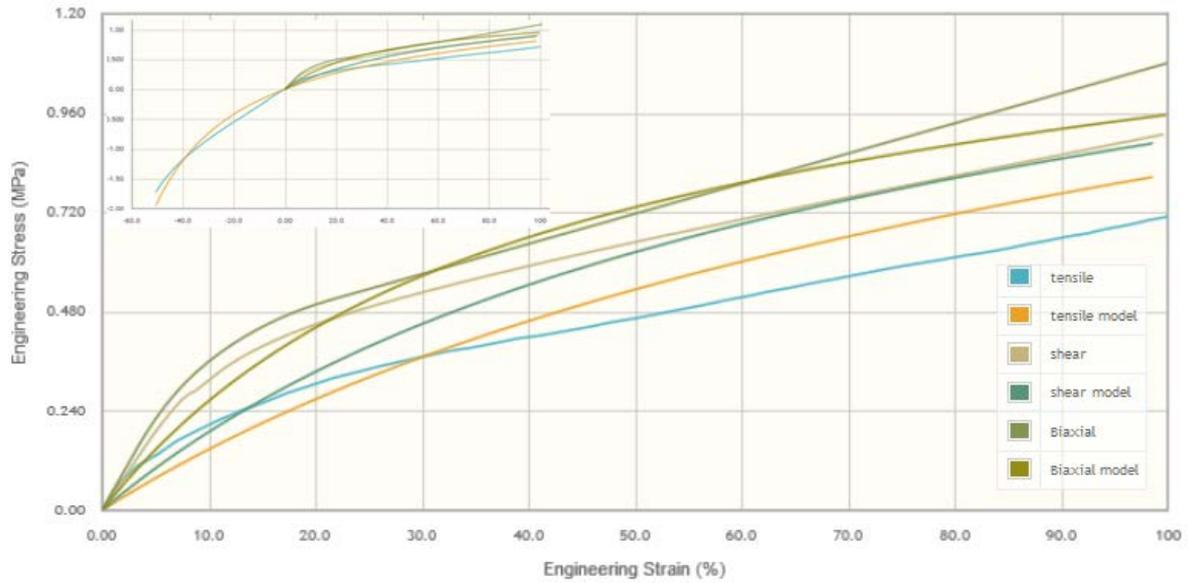
Figure 6 Ogden 3<sup>rd</sup> Order model plot of both data and model
