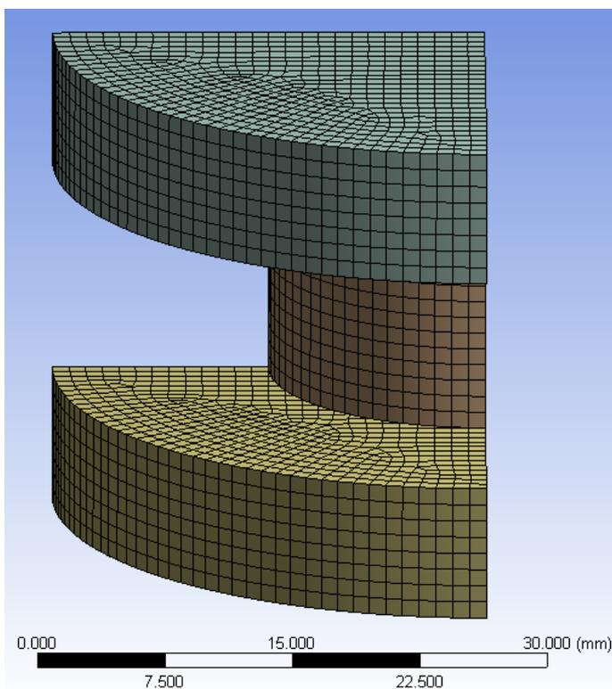
Figure 1 ANSYS Workbench quarter model of compression test.
