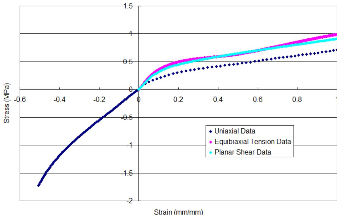
Figure 2 Stress-strain curves for Uniaxial, Equibiaxial, and Planar Shear data
