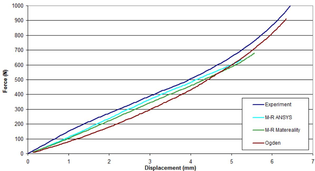
Figure 12 Validation for the mixed boundary condition also comparing several material models
