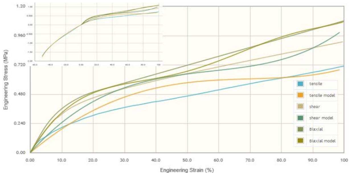
Figure 4: Mooney-Rivlin 9 parameter model plot of both data and model
