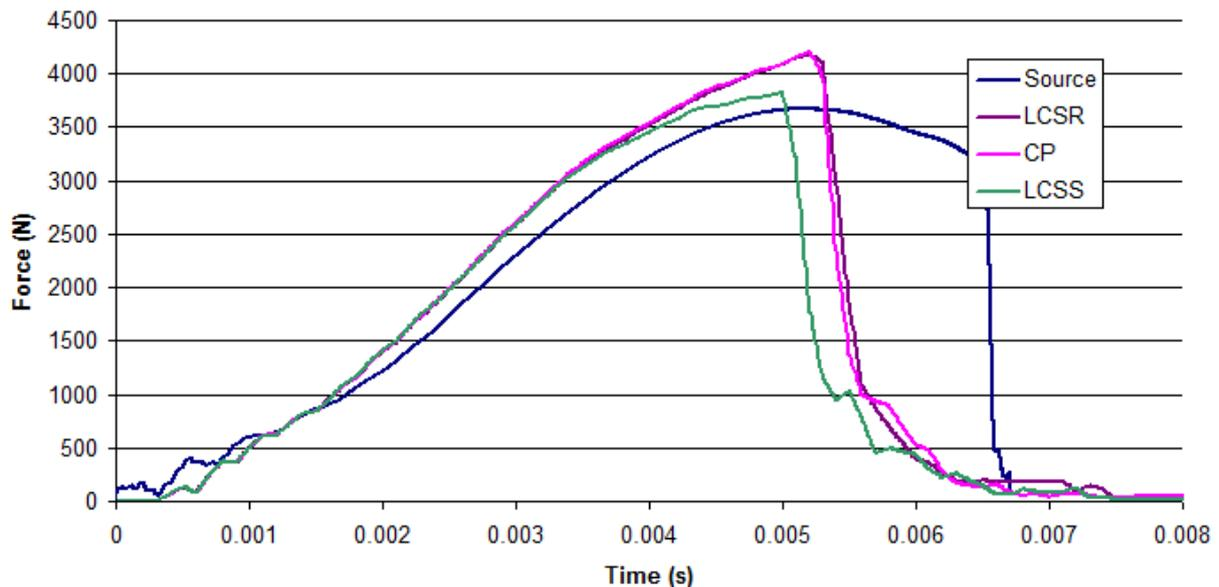
Fig.7: Falling dart (open loop) validation of MAT\_024 for ABS with visco-plasticity  $vp$  set to 1.
