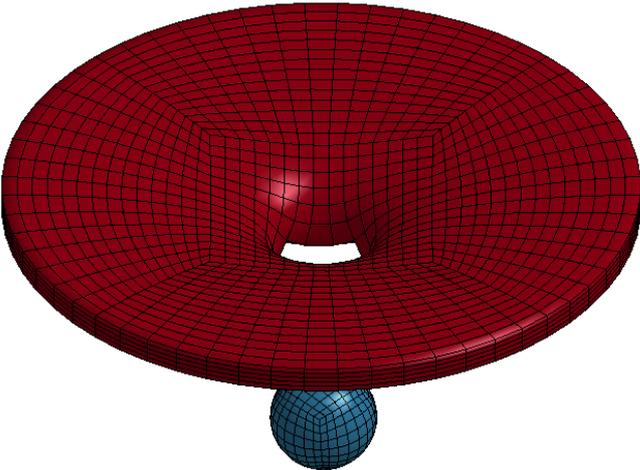
Fig.2: Falling dart impact simulation
