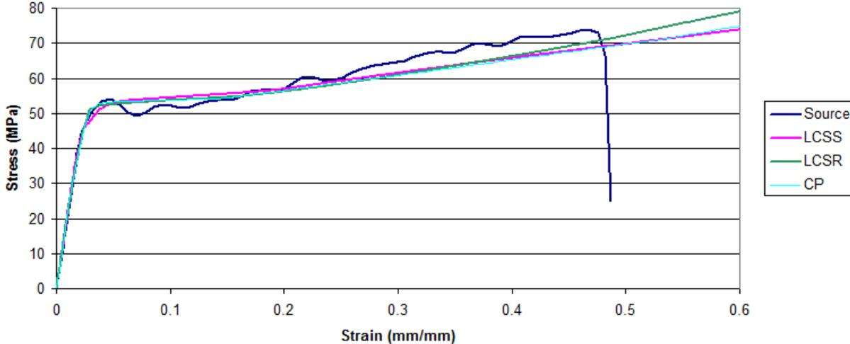
Fig.5: Closed loop validation of tensile test for ABS – MAT\_024- LCSS, LCSR, CP with  $vp=1$
