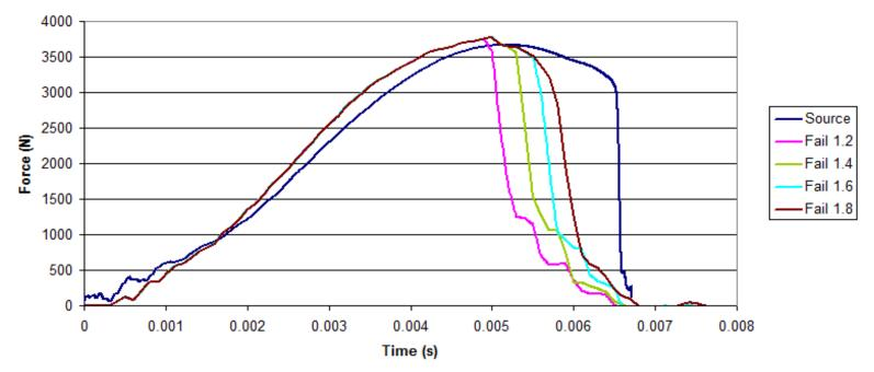
Starting around failure strains of 1.8 elements begin to be deleted for negative volume instead of hitting the failure strain
