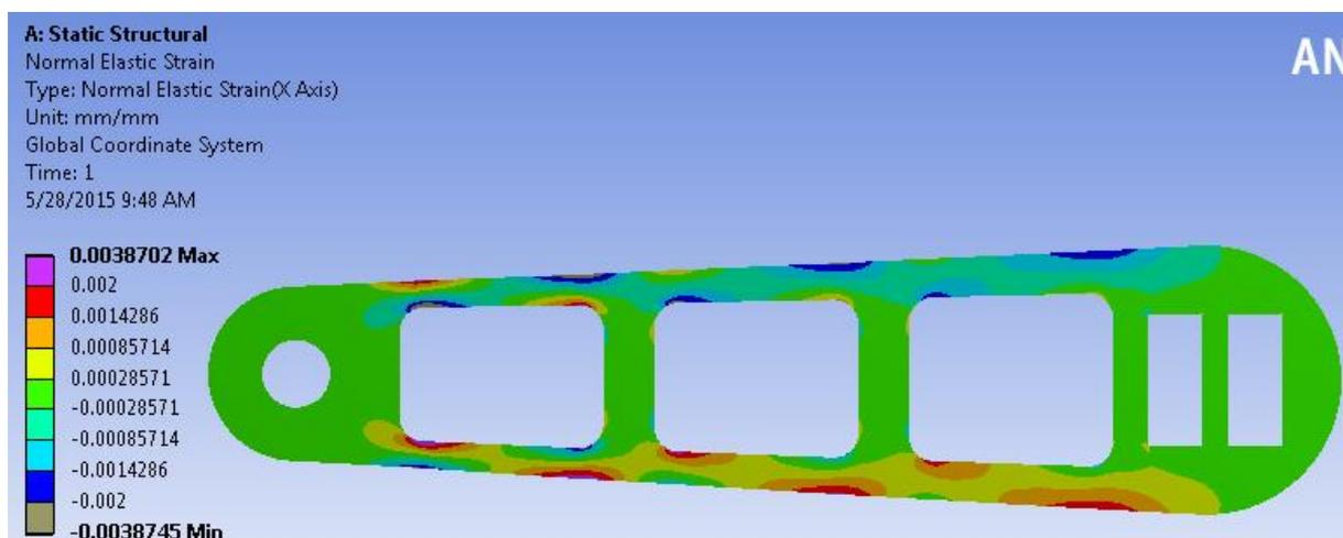
Figure 7 ANSYS x-strain contour with published modulus
