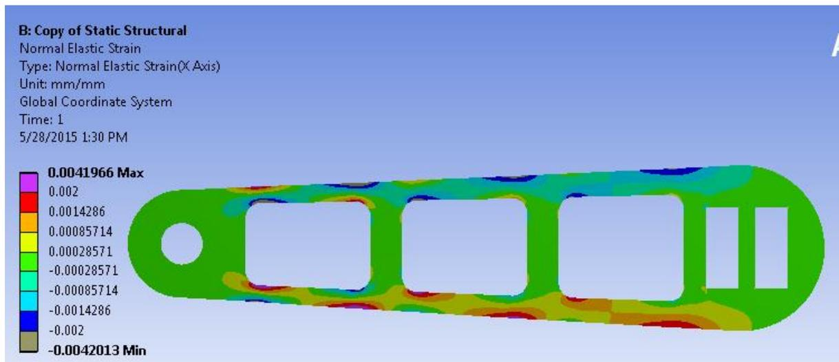
Figure 6 ANSYS x-strain contour with measured modulus
