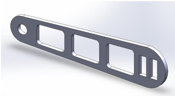
**Figure 1 Modified Cornell crank used in present work**
