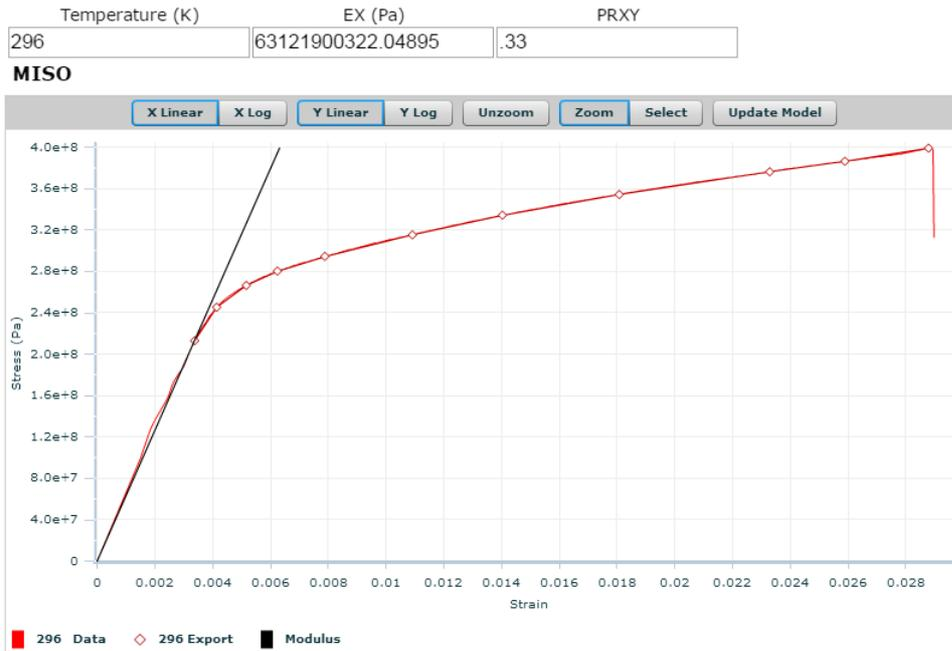
**Figure 8 90° orientation MISO Model created using Matereality CAE Modeler for ANSYS**
