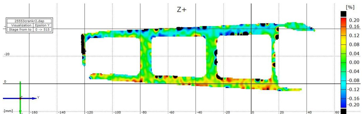
**Figure 5 Strain contour along the length of the crank**
