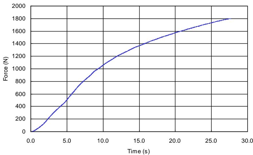
**Figure 9 Experimental force v time data for the crank until failure**
