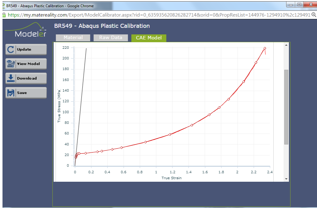
Figure 2: Goodness of fit plot for Abaqus elasto-plastic material model created using Matereality
