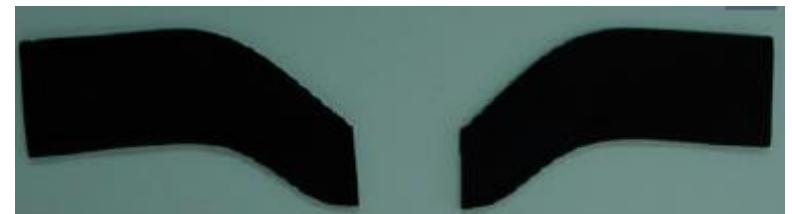
Failure mode during the tear test (ASTM D624 Type C Specimen)
