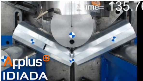
CAE correlation quasi-static 3-point bending tests. Courtesy of Faraday Future
